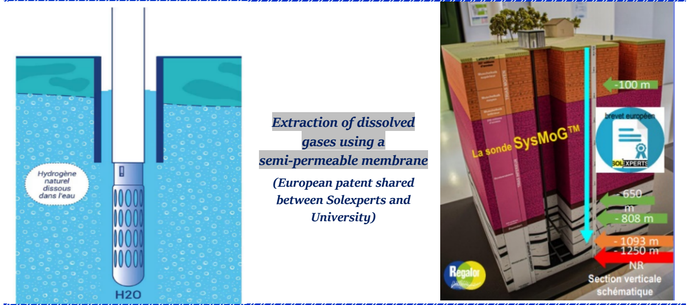
Fig. : A world-unique tool for measuring gases in boreholes
